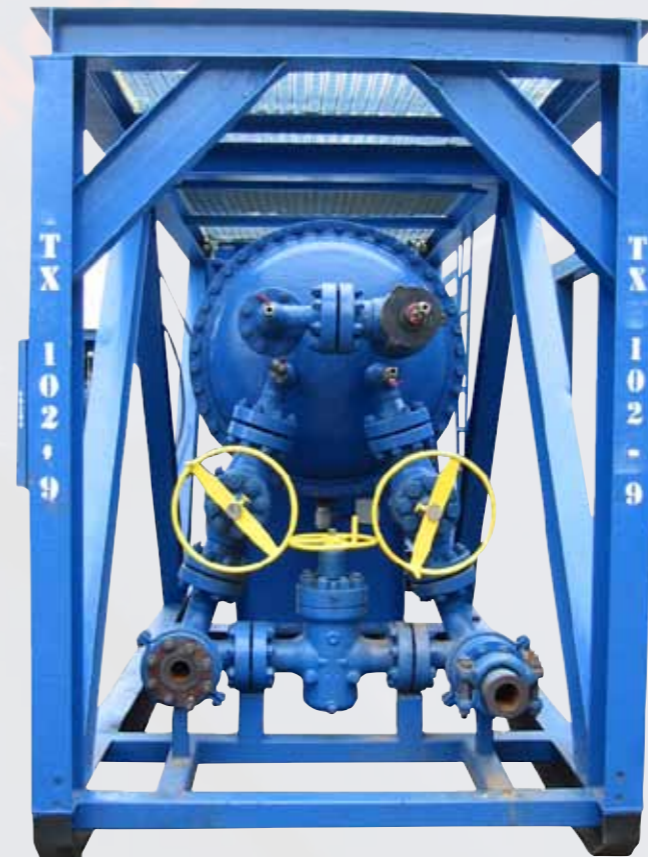
HEAT EXCHANGER – GATE VALVES
