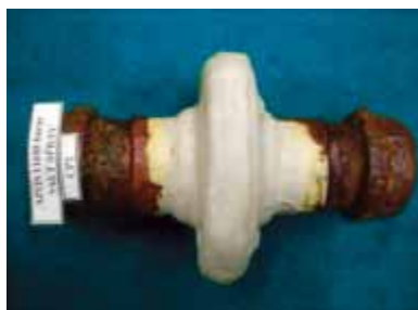
Flange with coating removed after 11,688 hours of salt spray test
