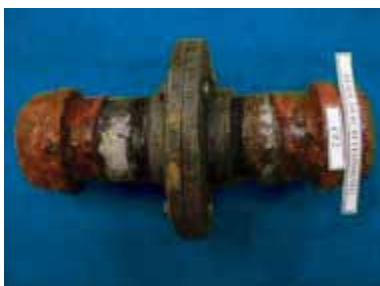
Absolute success after 11,688 hours of salt spray test
